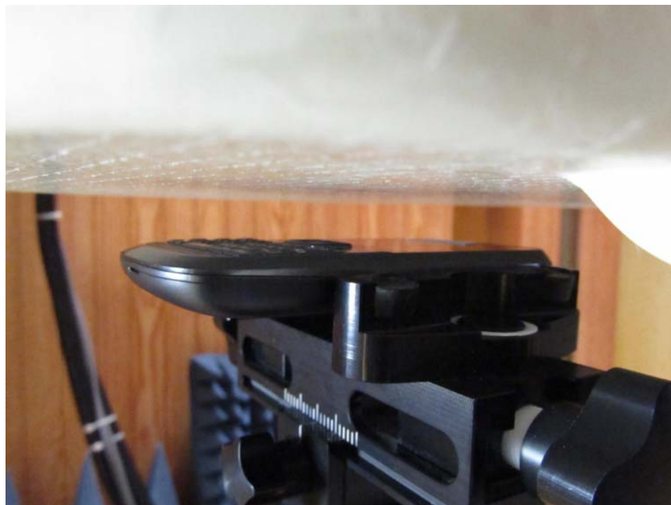
Figure 9E.4 FRONT Air Gap_15mm
