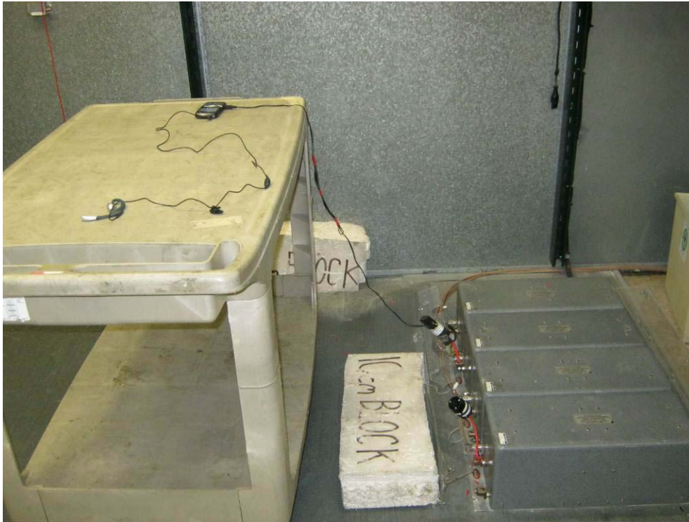
Figure 1 Test Setup for Conducted Emissions
