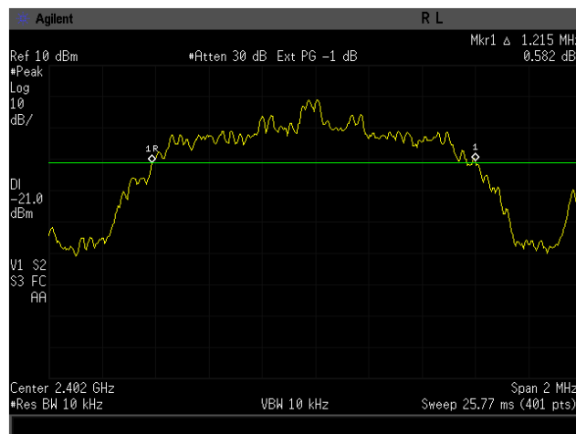
Figure 6-1c: 20dB Bandwidth EDR D8PSK, Channel 0.
