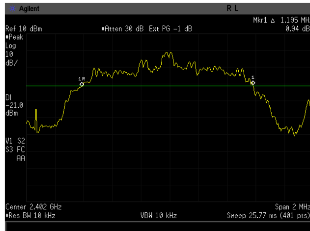
Figure 6-1b: 20dB Bandwidth EDR DQPSK, Channel 0.
