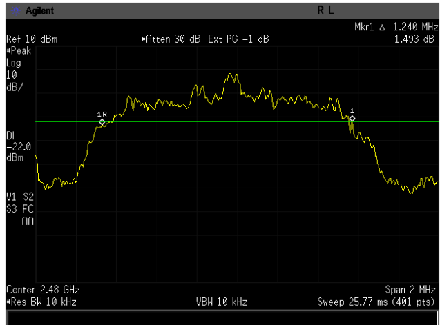
Figure 6-3b: 20dB Bandwidth EDR DQPSK, Channel 78.
