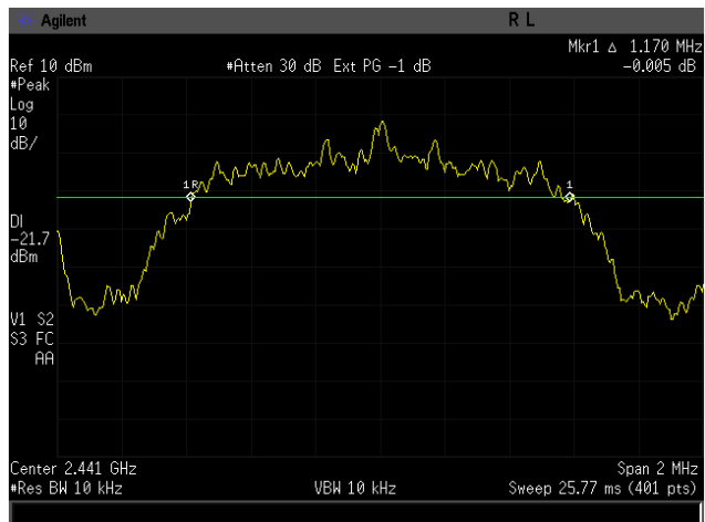
Figure 6-2c: 20dB Bandwidth EDR D8PSK, Channel 39.
