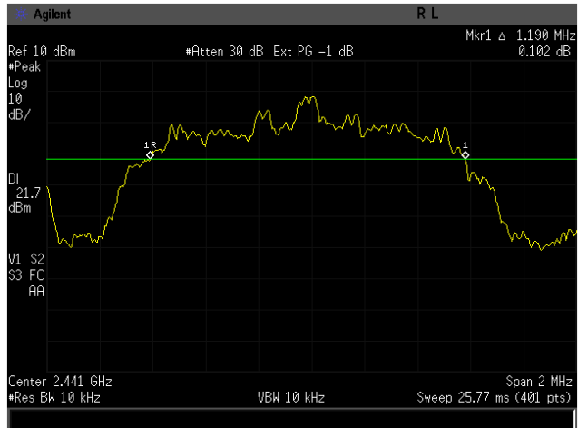
Figure 6-2b: 20dB Bandwidth EDR DQPSK, Channel 39.
