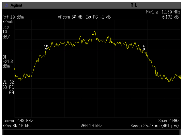
Figure 6-3c: 20dB Bandwidth EDR D8PSK, Channel 78.
