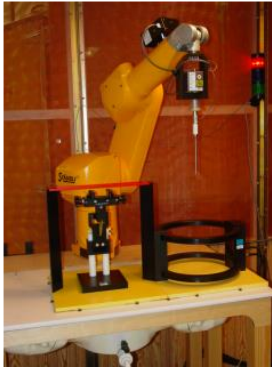
Figure 4.2a T-Coil setup with Helmholtz Coil
