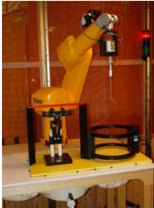
Figure 4.2a T-Coil setup with Helmholtz Coil
