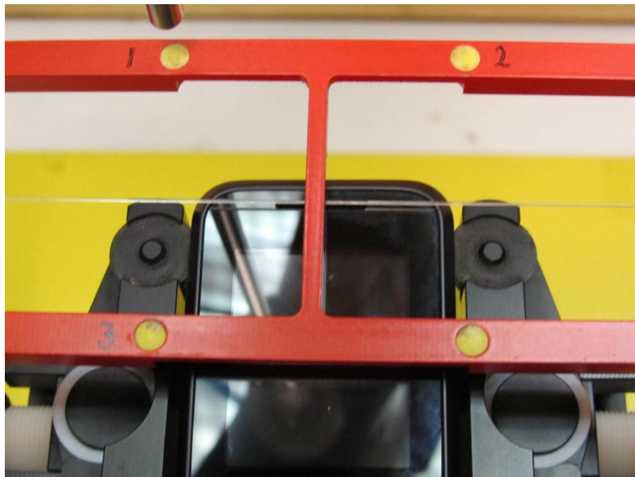
Figure 1b – HAC Tcoil Emission Test Setup
