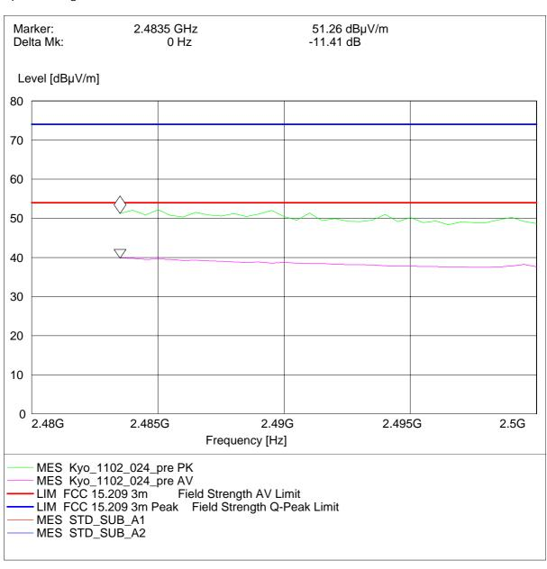
Radiated measurement (higher band edge)
