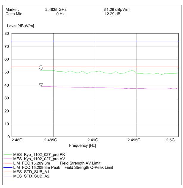
Radiated measurement (higher band edge)
