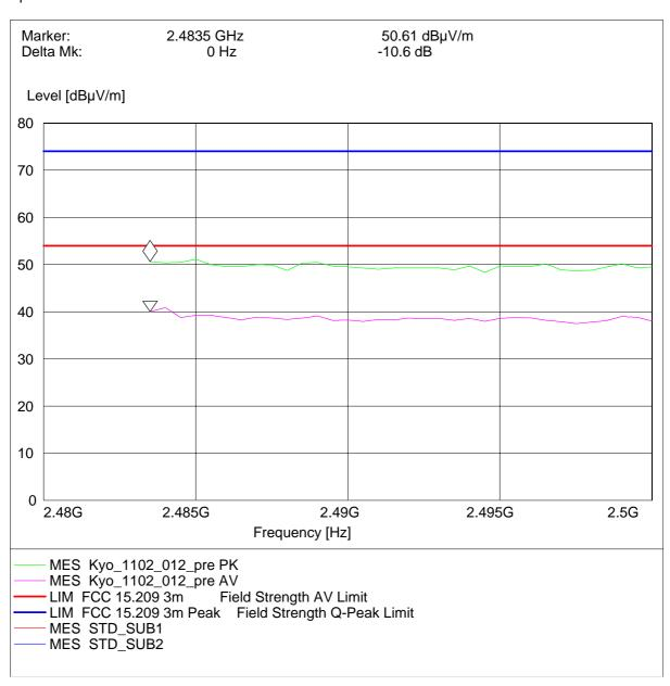
Radiated measurement (higher band edge)
