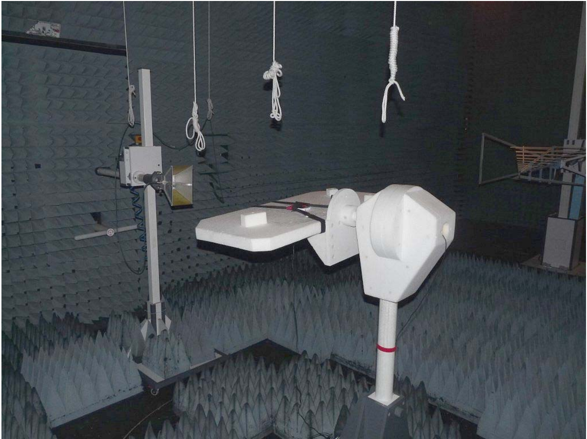
Photo 3: Test setup for radiated measurements in fully anechoic chamber used for: FCC Part 15 (Enclosure, above 1 GHz up to 18 GHz) Note: For measurements 18-25 GHz the horn antenna is replaced by an appropriate horn antenna (not shown at the photo). FCC Part 24 (Enclosure, above 30 MHz up to 20 GHz).
