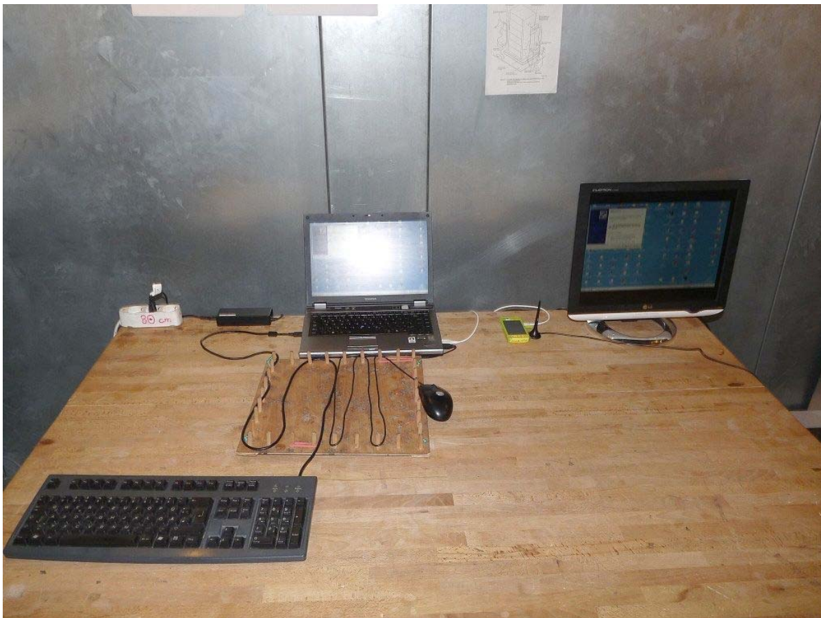
Photo 5: Test setup for conducted measurements (AC Port (power line)); computer peripheral setup, supplied by computer
