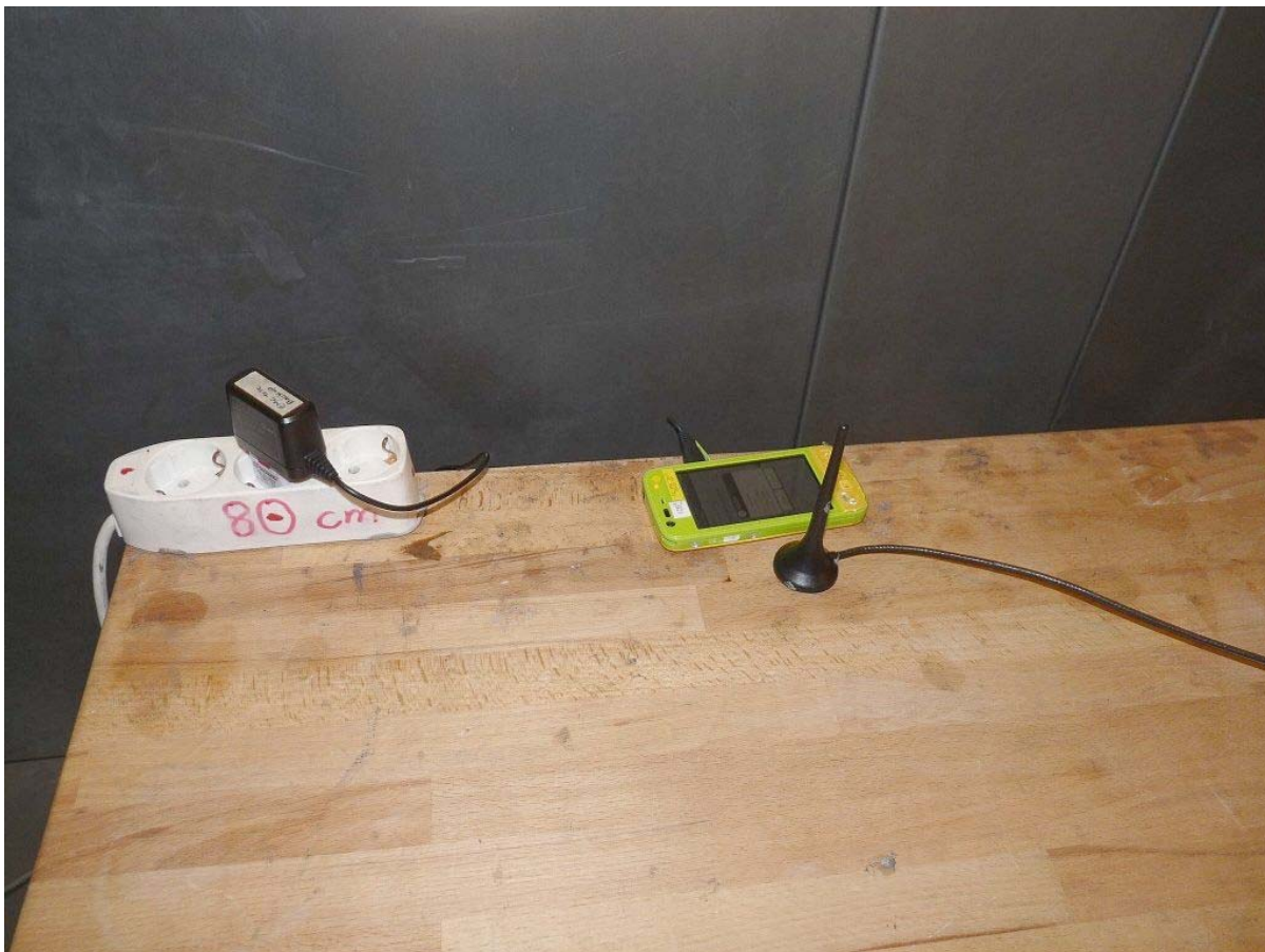
Photo 4: Test setup for conducted measurements (AC Port (power line)); supplied by AC/DC adapter
