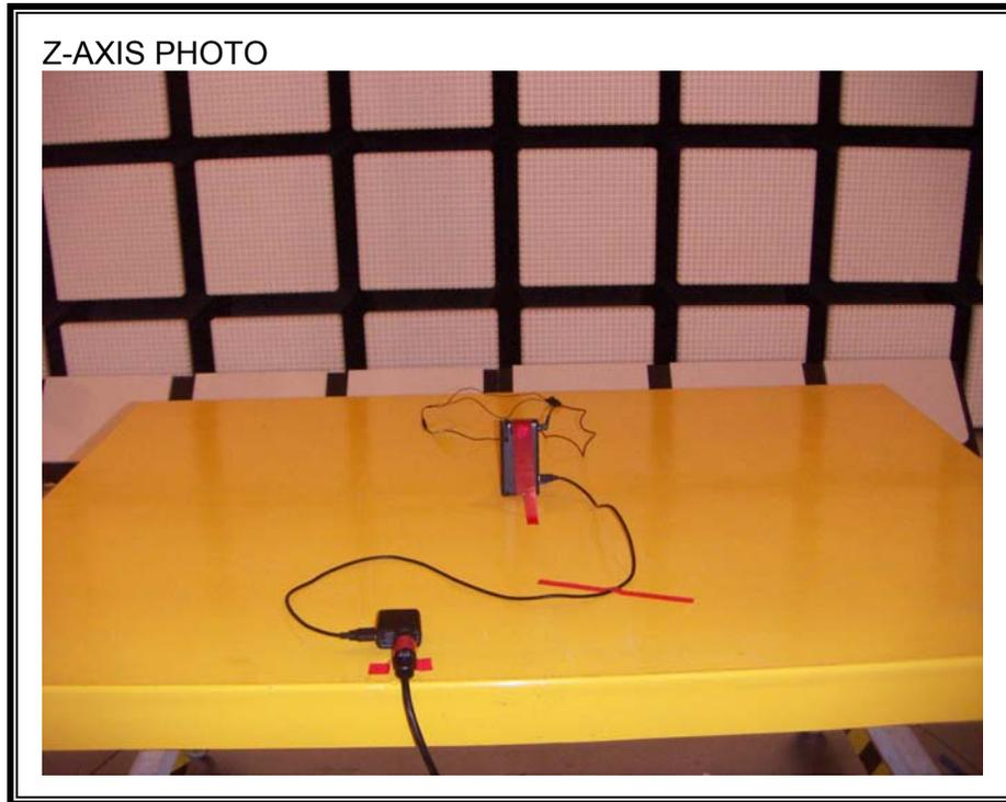
**POWER-LINE CONDUCTED EMISSIONS MEASUREMENT SETUP**
