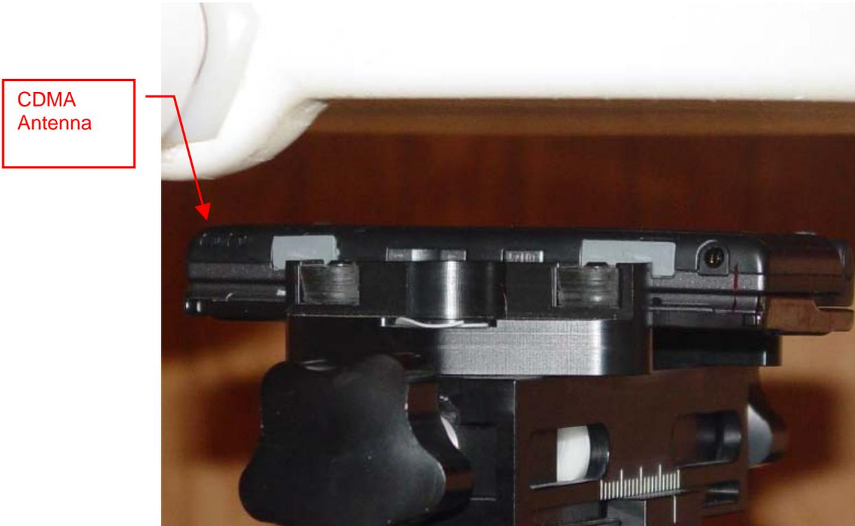
**Figure 9E.11** Body SAR setup (Closed, Face Down "Back"), 22mm Air Separation)
