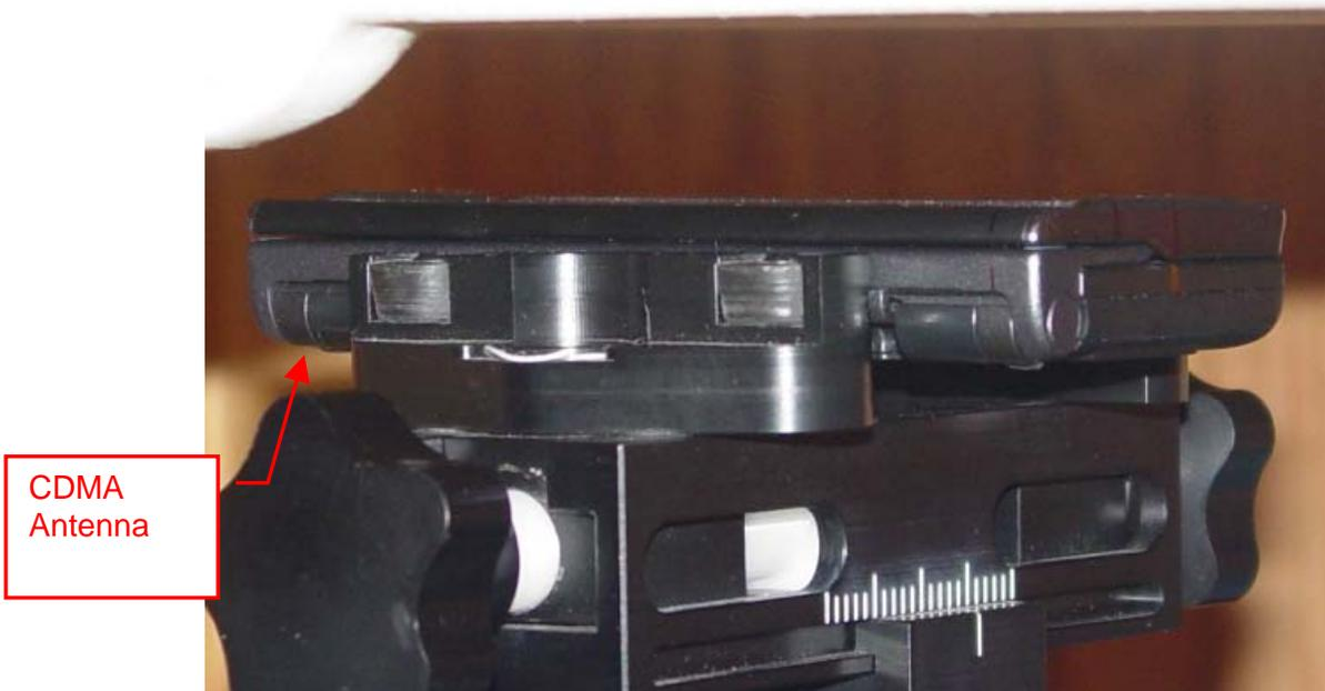
**Figure 9E.14** Body SAR setup (Closed, Face Up), 22mm Air Separation)
