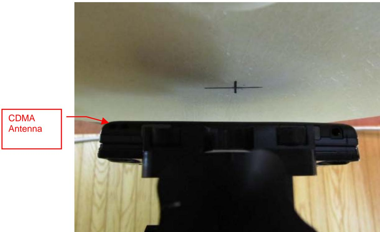
**Figure 9E.12** Body SAR setup (Closed, Face down "Back", 22mm Air Separation)\_Front view
