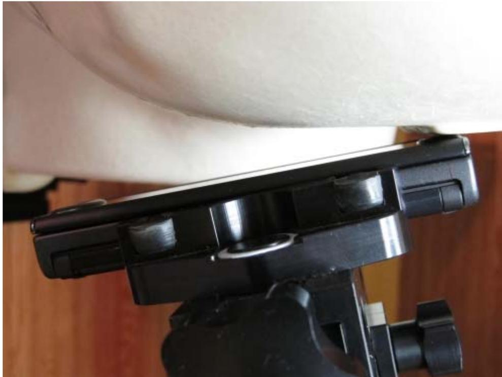
**Figure 9E.4** Phone (Closed) against the head (Left Tilt position)
