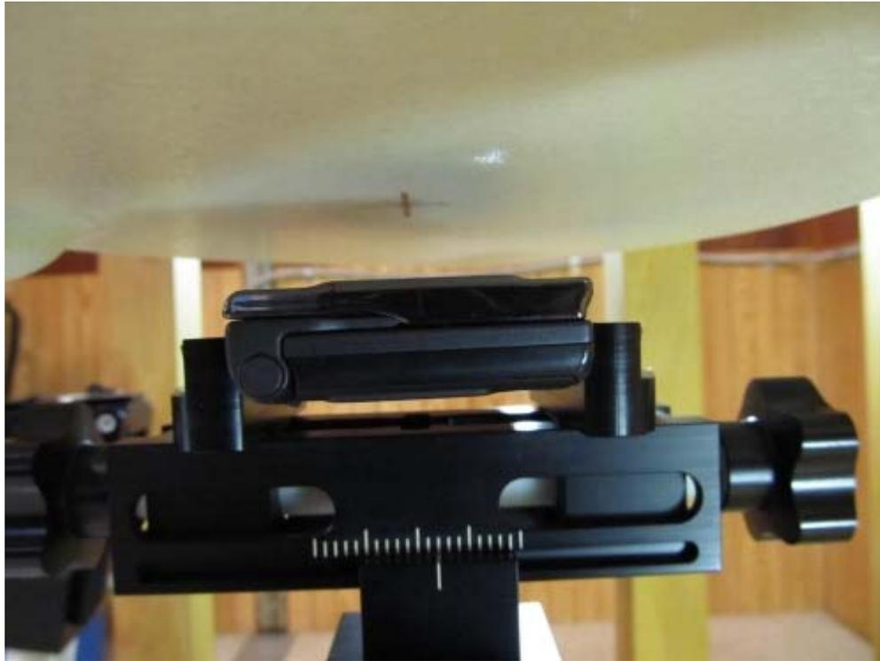
**Figure 9E.13** Body SAR setup (Closed, Face Up "Top", 22mm Air Separation)\_Side view
