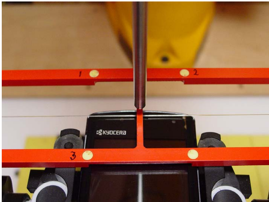
Figure 1b – HAC T-Coil Test Setup
