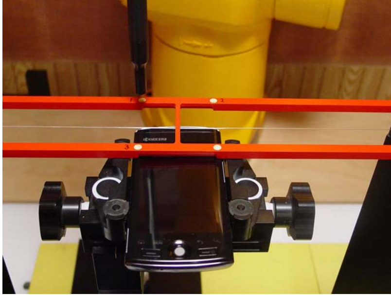
Figure 1a – HAC RF Emission Test Setup
