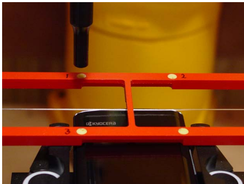
Figure 1b – HAC RF Emission Test Setup
