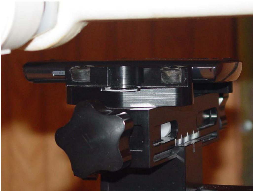
Figure 9E.4 Body SAR setup (Face Up, 22mm Air Separation)
