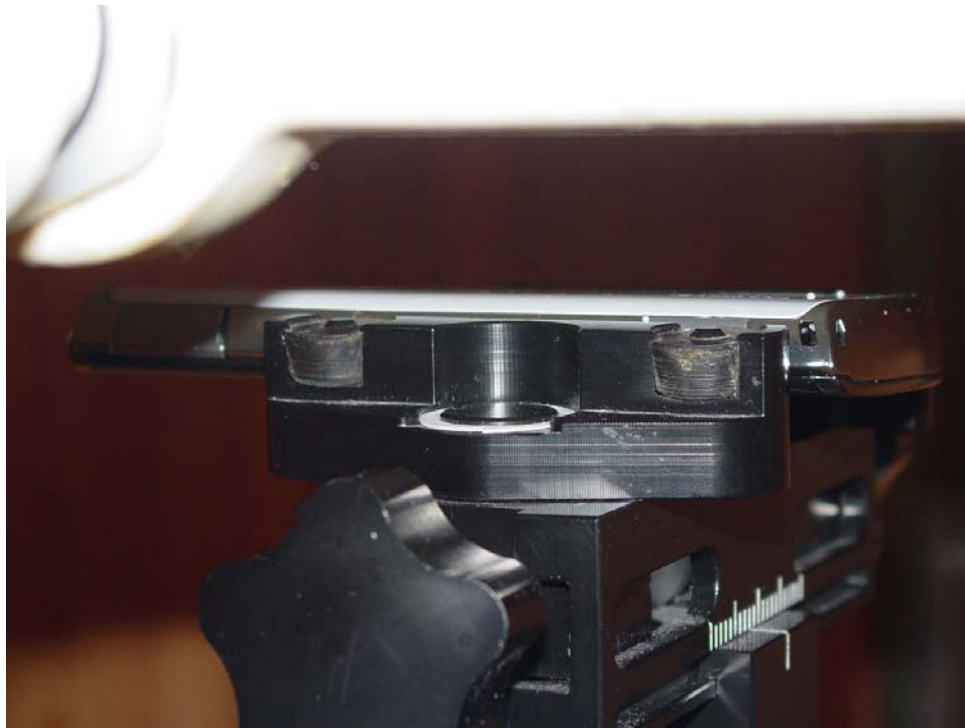
Figure 9E.3 Body SAR setup (Face Down, 22mm Air Separation)
