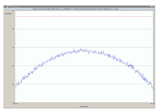
Test: 22.1; Frequency Band = 850, Mode = GSM, Channel = 128, Frequency = 824.2MHz, Method = conducted
