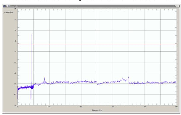
Test: 22.3; Frequency Band = 850, Mode = GSM, Channel = 128, Frequency = 824.2MHz,
