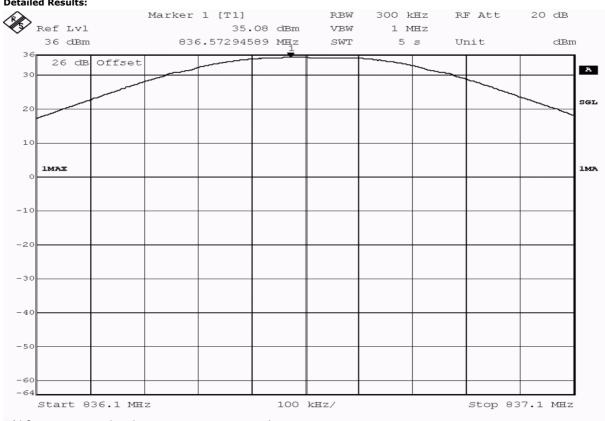
output power measurement DE020, GSM850, output power, channel 190, Comment A:
