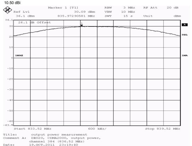
Test: 22.1; Frequency Band = 800, Mode = CDMA2000, Channel = 384, Frequency = 836.5MHz, Method = radiated
