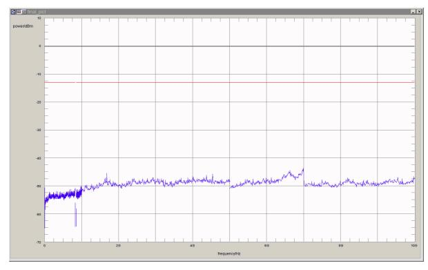
Test: 22.3; Frequency Band = 800, Mode = CDMA2000, Channel = 777, Frequency = 848.3MHz
