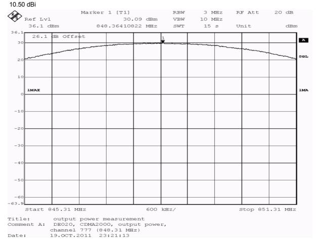
Test: 22.1; Frequency Band = 800, Mode = CDMA2000, Channel = 777, Frequency = 848.3MHz, Method = radiated
