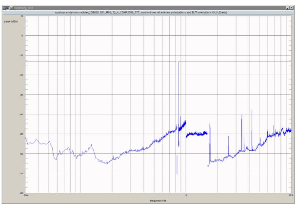
Test: 22.4; Frequency Band = 850, Mode = GSM, Channel = 128, Frequency = 824.2MHz
