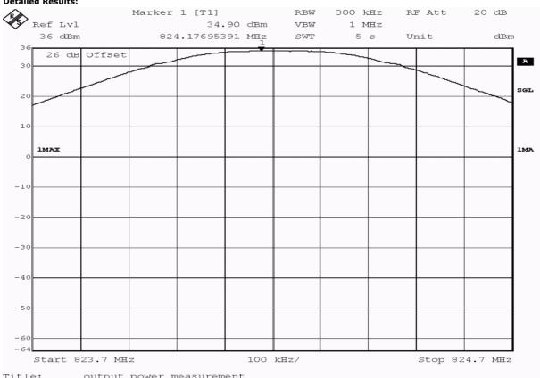
output power measurement DE020, GSM850, output power, channel 128, Comment A:
