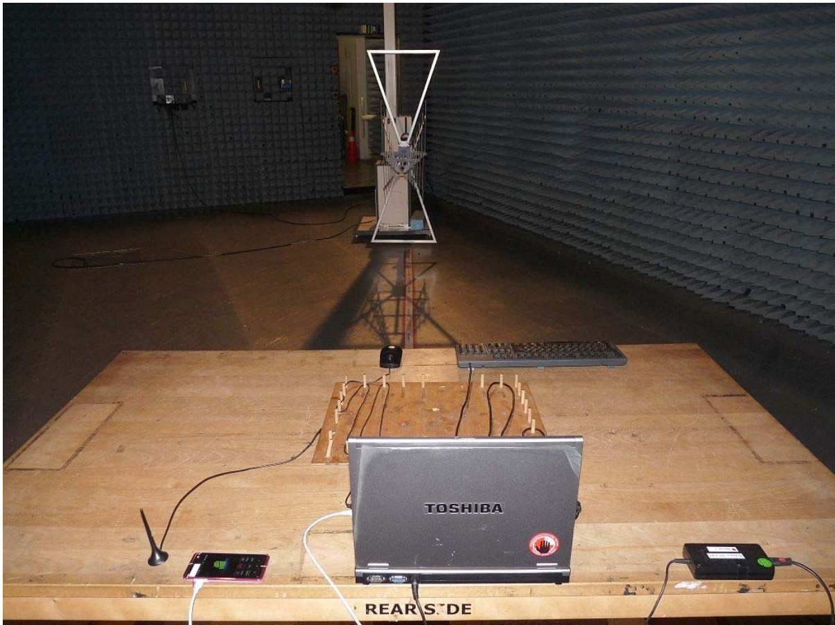
Photo 6: Test setup for radiated measurements (unintentional transmission); computer peripheral setups PC_V02 and PC2_V02, the WLAN access point is not visible because it is placed outside of the semi-anechoic chamber
