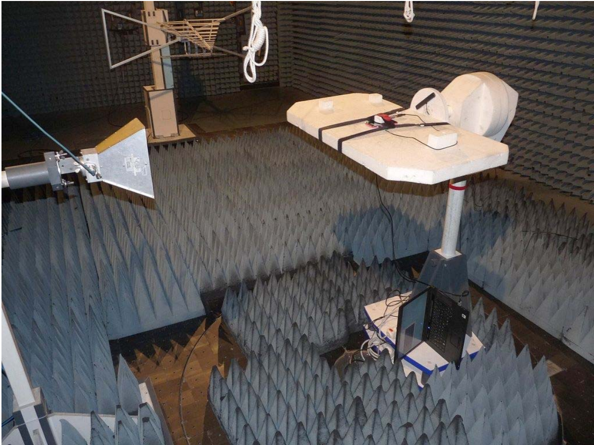
Photo 3: Test setup for radiated measurements (Enclosure, above 1 GHz up to 18 / 20 GHz)
