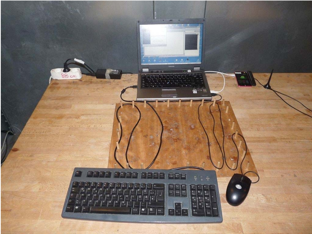
Photo 5: Test setup for conducted measurements (AC Port (power line)); computer peripheral setups PC_V02 and PC2_V02, the WLAN access point is not visible because it is placed outside of the shielded room
