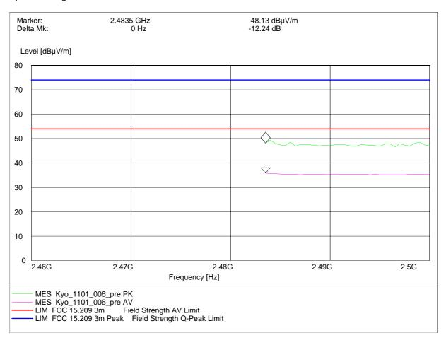
Radiated measurement (higher band edge)
