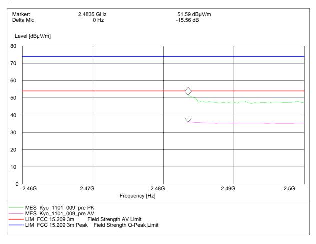
Radiated measurement (higher band edge)
