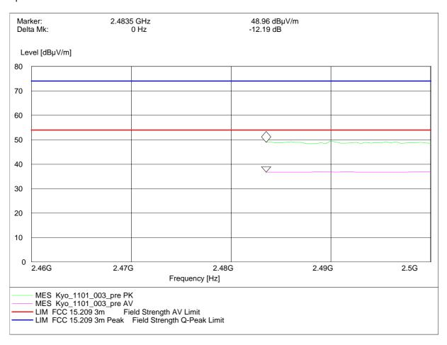
Radiated measurement (higher band edge)
