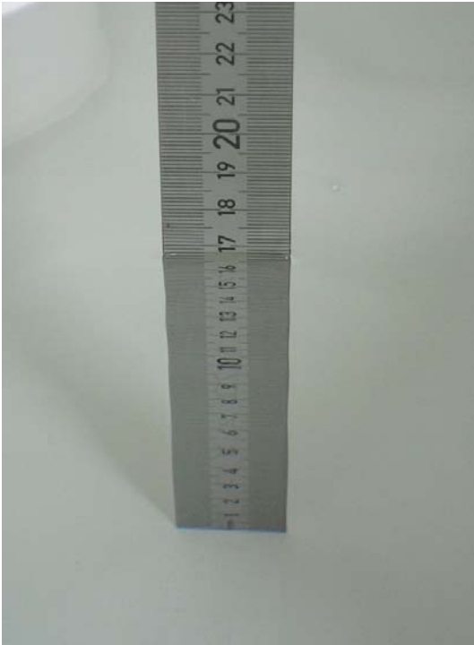
Fig. 38: Liquid depth for IEEE 802.11 Body measurements
