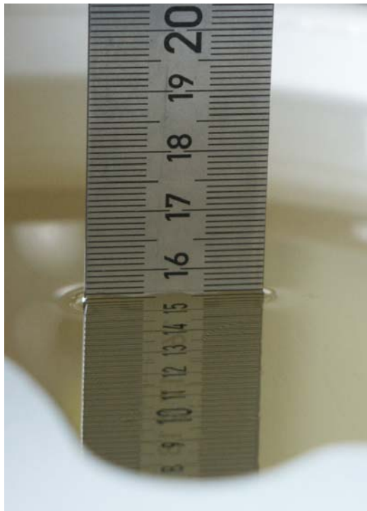
Fig. 34: Liquid depth for GSM/GPRS 850 and CDMA 2000 Head measurements
