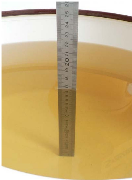
Fig. 36: Liquid depth for GSM/GPRS 850 and CDMA 2000 body measurements.
