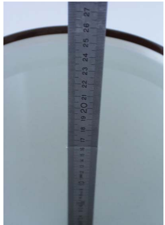
Fig. 35: Liquid depth for PCS 1900 Head measurements
