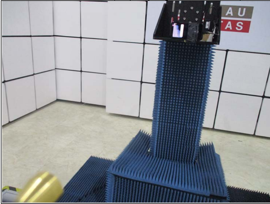
Radiated Emission Test (Frequency range 110GHz ~ 170GHz)
