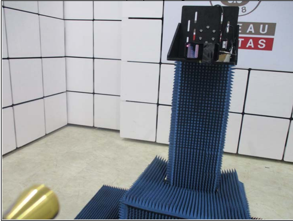
Radiated Emission Test (Frequency range 75GHz ~ 110GHz)
