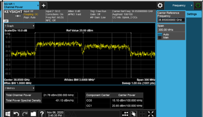
2CC / QPSK / Mid Channel
