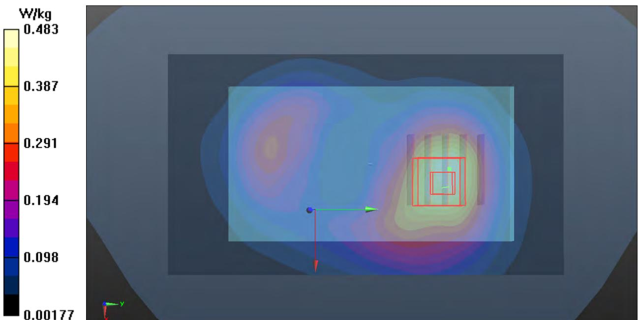
**P353 LTE 25\_QPSK\_10M\_Rear Face\_1cm\_Ch26365\_1RB\_offset 0\_Earphone****DUT: 121012C09**
