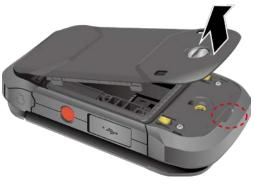
3. Insert the battery, making sure to align the gold contacts (1). Press down gently to secure the battery (2).
