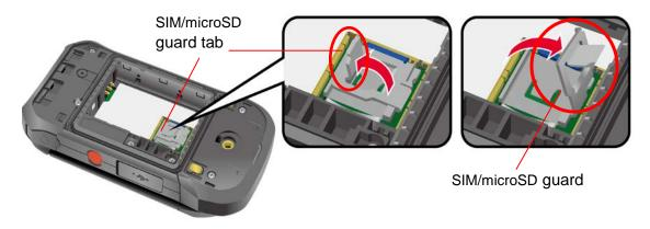
3. Slide the microSD card into the slot with the gold contacts facing down. Gently push the card in until it fits into place.
