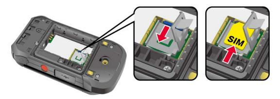
**Note:** Please be careful to not insert the SIM card into the SD card slot.
