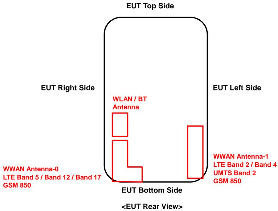
The separation distance for antenna to edge:
