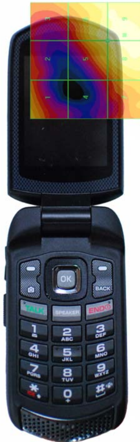
Figure 18-4 E-Field WD Scan overlay (T-Coil Centered Scan Pictured)
