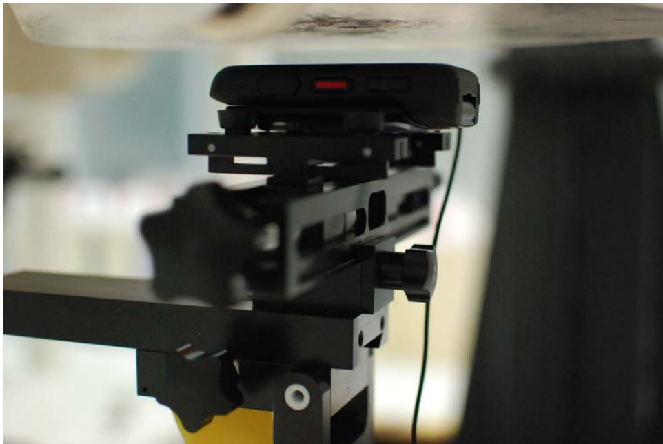
SAR Test Setup Photo 8 – Body-Worn Back Side at 15 mm with Headphones Accessory
