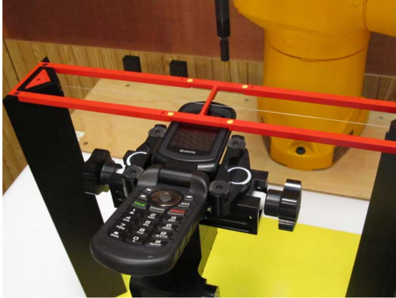
Figure 1a – HAC RF Emission Test Setup
