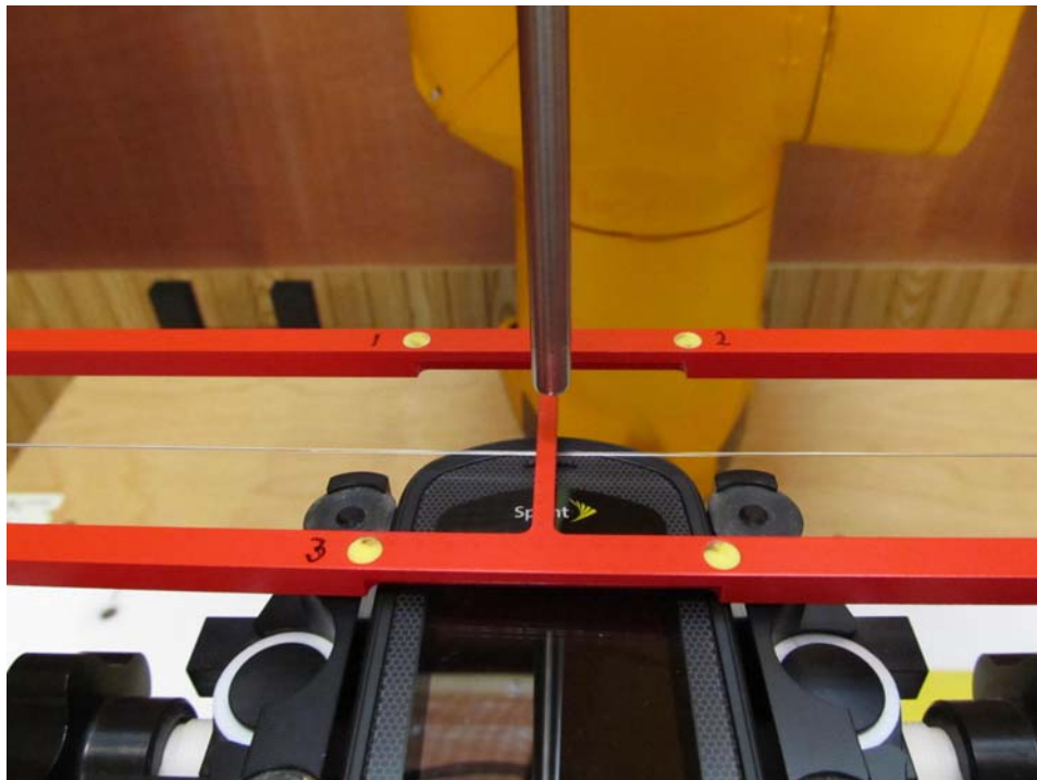
Figure 1b – HAC T-Coil Test Setup
