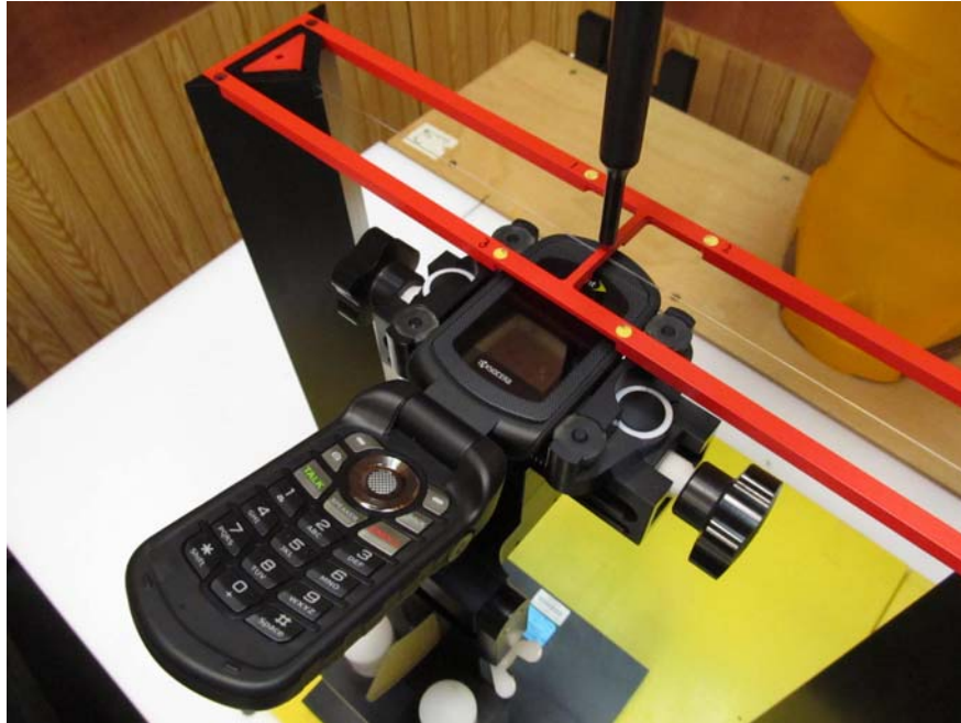
Figure 1a – HAC RF Emission Test Setup
