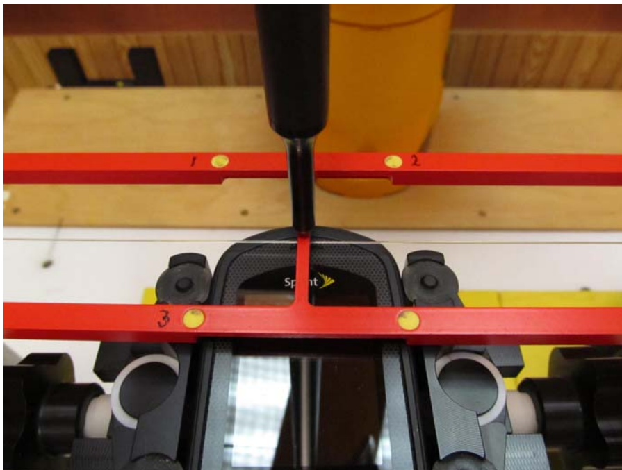
Figure 1b – HAC RF Emission Test Setup
