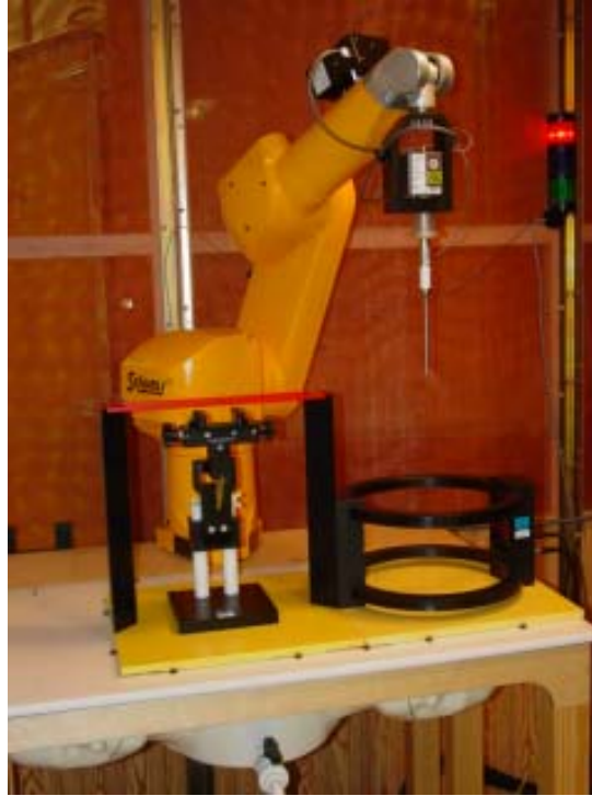
Figure 4.2a T-Coil setup with Helmholtz Coil
