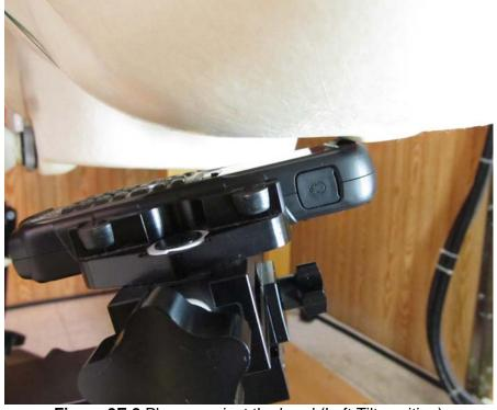
Figure 9E.2 Phone against the head (Left Tilt position)
