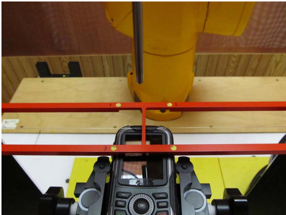
Figure 1b – HAC T-Coil Test Setup
