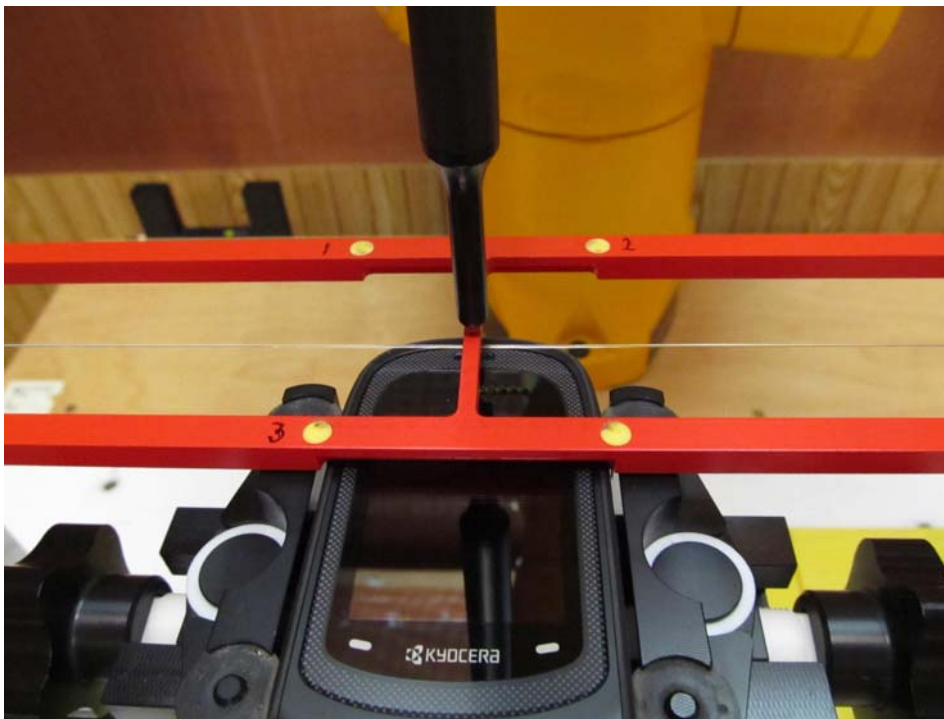
Figure 1b – HAC RF Emission Test Setup
