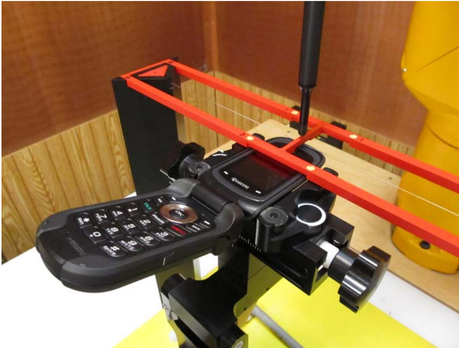
Figure 1a – HAC RF Emission Test Setup
