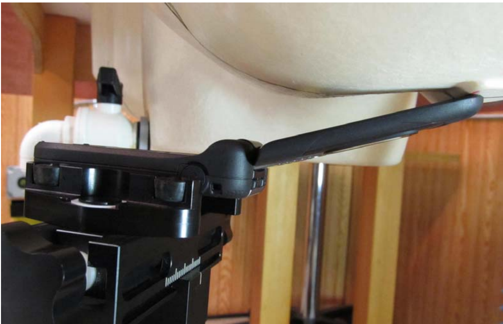
Figure 9E.2 Phone against the head (Left Tilt position)
