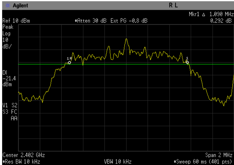
Figure 6-1b: 20dB Bandwidth EDR DQPSK, Channel 0.
