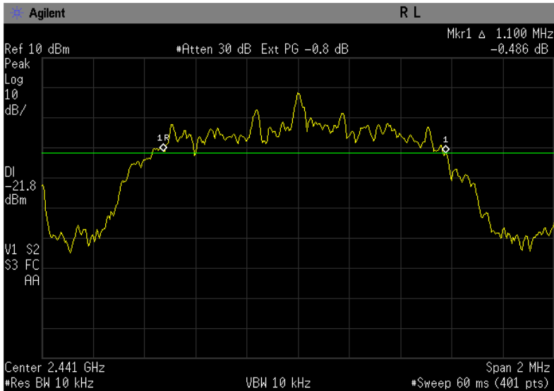
Figure 6-2b: 20dB Bandwidth EDR DQPSK, Channel 39.
