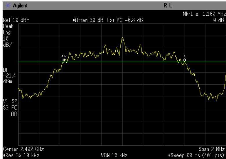
Figure 6-1c: 20dB Bandwidth EDR D8PSK, Channel 0.
