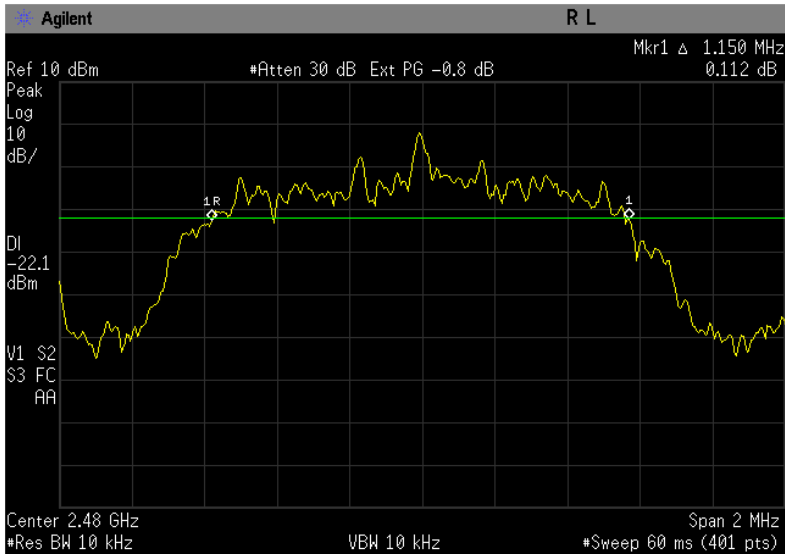
Figure 6-3b: 20dB Bandwidth EDR DQPSK, Channel 78.
