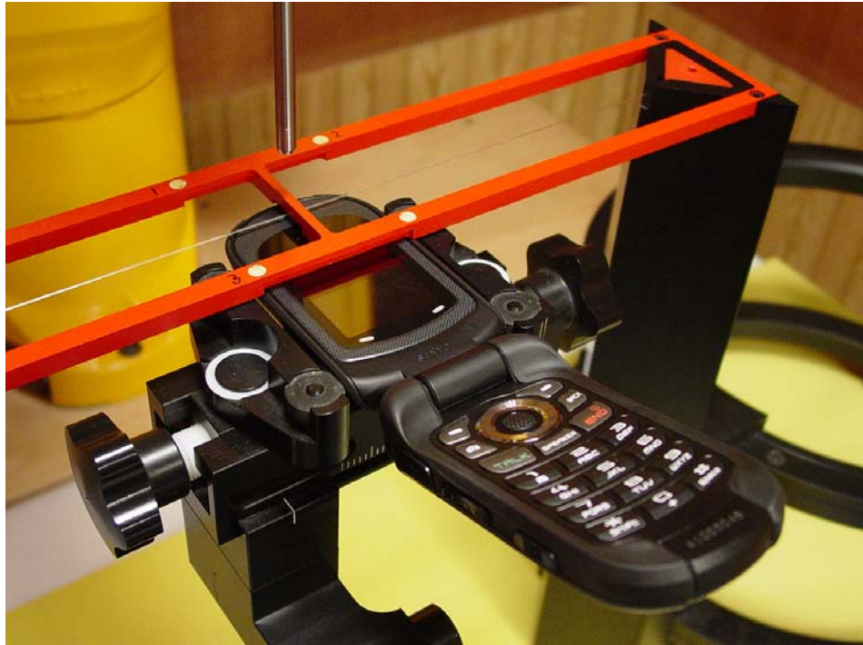
Figure 1a – HAC T-Coil Test Setup
