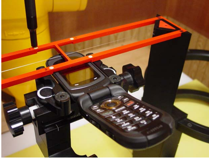
Figure 1a – HAC RF Emission Test Setup
