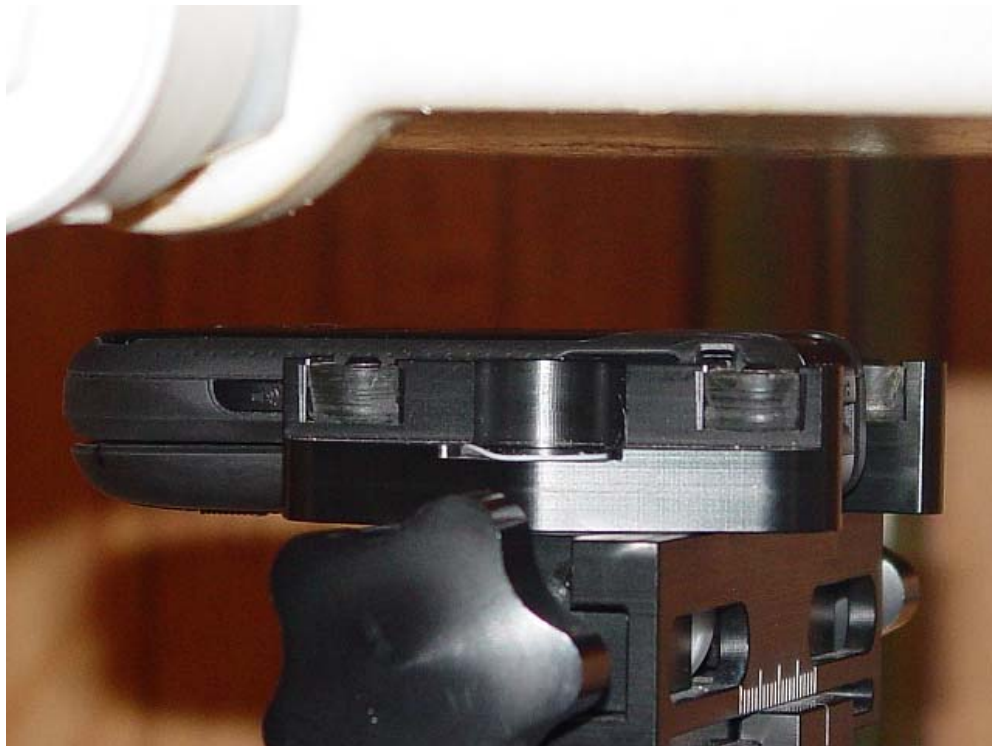
Figure 9E.4 Body SAR setup (Closed, Face Down, 22mm Air Separation)
