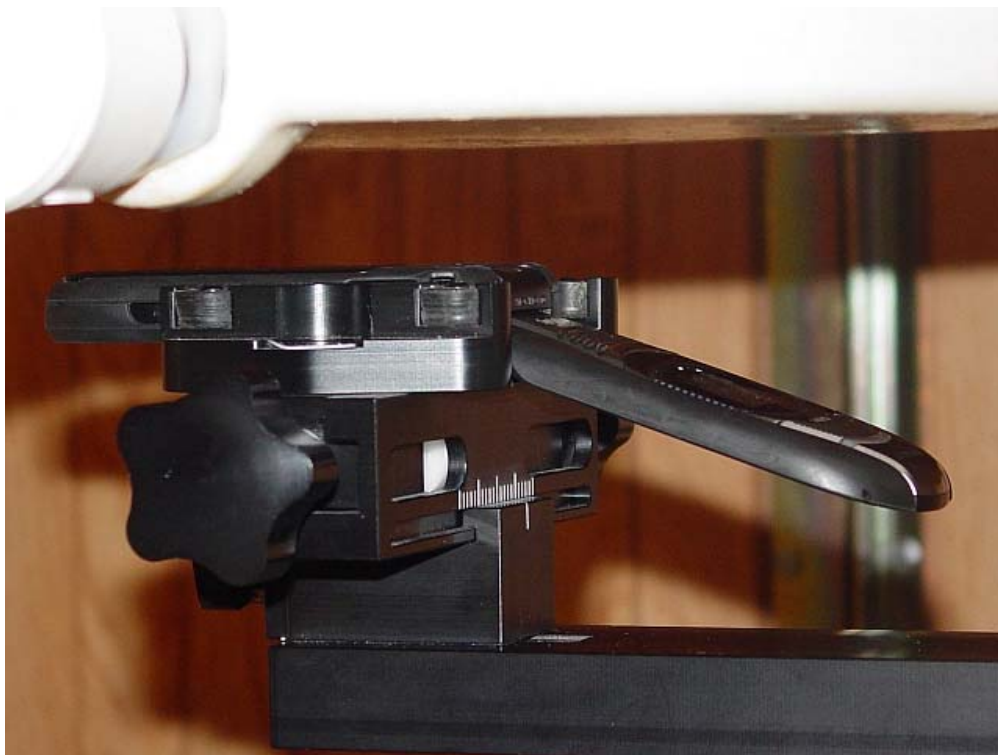
Figure 9E.6 Body SAR setup (Open, Face Down, 22mm Air Separation)
