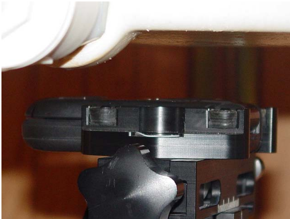
Figure 9E.5 Body SAR setup (Closed, Face Up, 22mm Air Separation)
