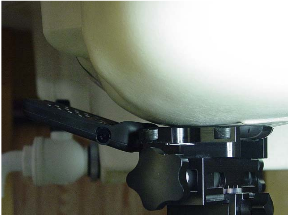
Figure 9E.1 Phone (Open) against the head (Left cheek position)
