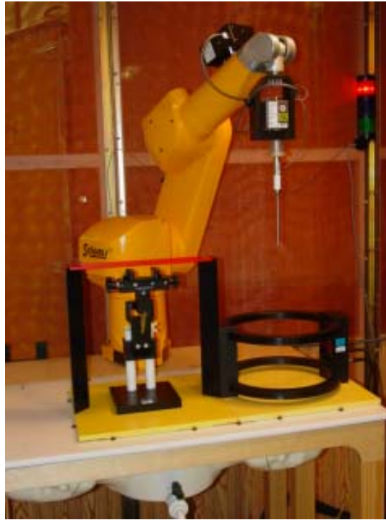
Figure 4.2a T-Coil setup with Helmholtz Coil
