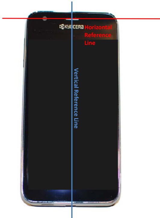
SAR Test Setup Photo 11 – DUT Reference Lines
