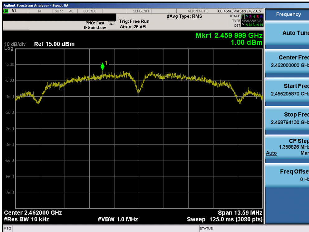
Plot 6-12. Power Spectral Density Plot (802.11b – Ch. 11)
