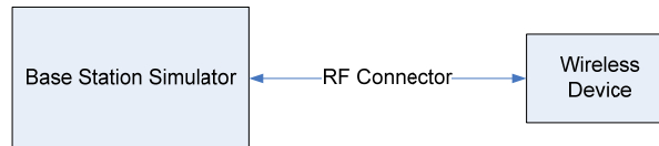
Figure 9-1 Power Measurement Setup
