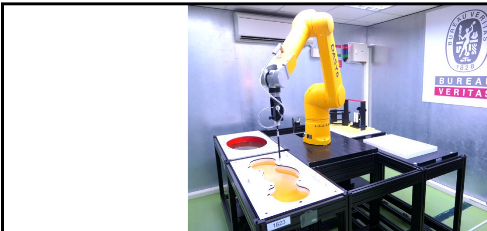
Fig-3.2 SPEAG DASY6 System
