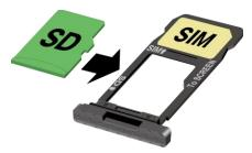
**NOTE:** If you need to reinstall your SIM card, remove the original SIM card from the tray and place your new SIM card into the tray with the gold contacts facing down as shown.
