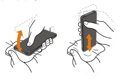
3. After removing all the water, let the phone dry completely at room temperature.
