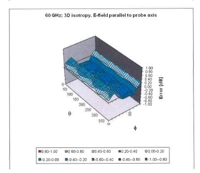
Probe isotropy for  $E_{tot}$ : probe rotated  $\varphi = 0^{\circ}$  to 360°, tilted from field propagation direction  $\vec{k}$ Parallel to the field propagation ( $\psi = 0^{\circ} - 90^{\circ}$ ) at 30 GHz: deviation within ± 0.38 dB Parallel to the field propagation ( $\psi = 0^{\circ} - 90^{\circ}$ ) at 60 GHz: deviation within ± 0.40 dB
