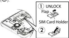
3. Insert the nano SIM card into the flap of the SIM card holder, making sure the cut-off corner is at the top right and the card is inserted behind the SIM guide tabs(3).
