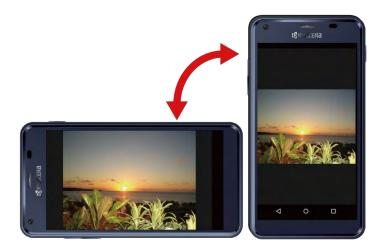
Note: The Auto-rotate check box needs to be selected for the screen orientation to automatically change.
