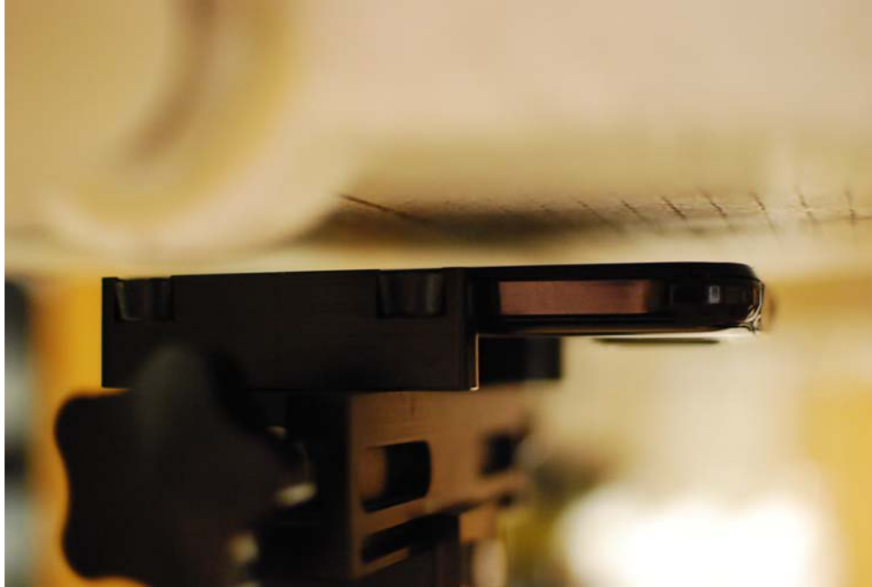
SAR Test Setup Photo 3: Front Side at 10 mm
