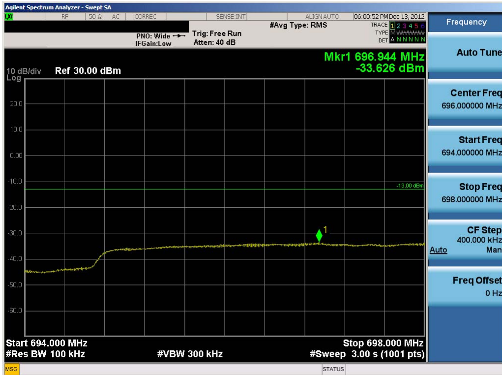
Plot 7-26. Lower Extended Band Edge Plot (5.0MHz QPSK – RB Size 25)
