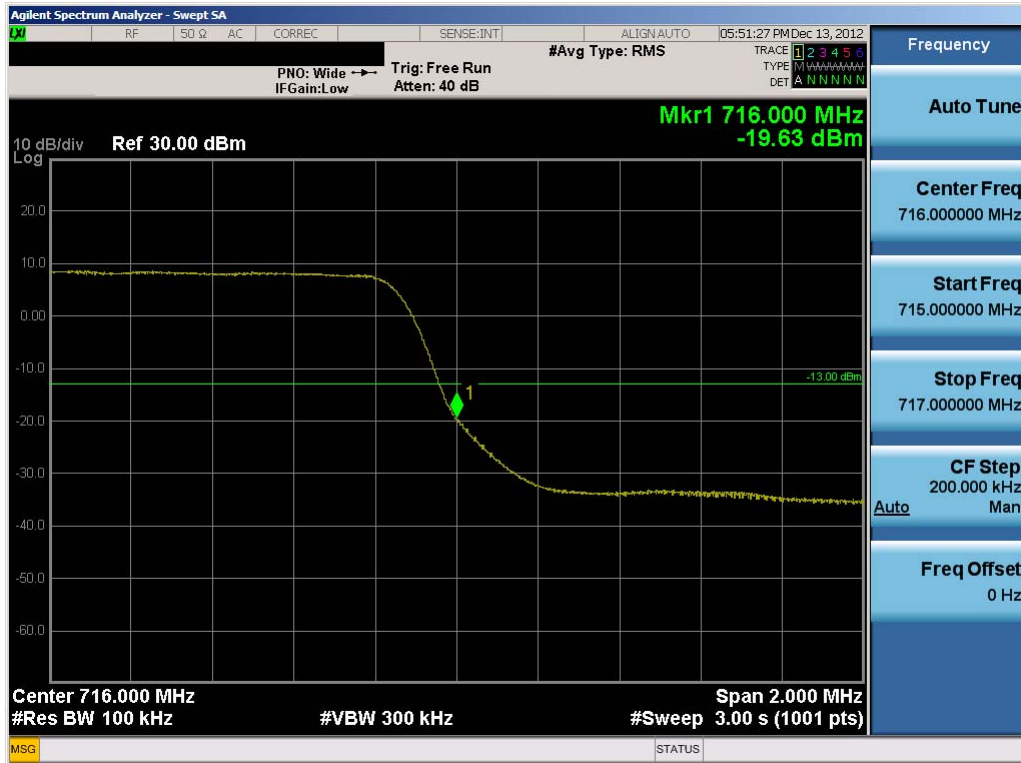
Plot 7-23. Upper Band Edge Plot (3.0MHz QPSK – RB Size 15)
