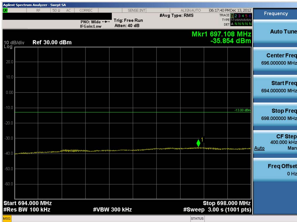
Plot 7-38. Lower Extended Band Edge Plot (10.0MHz QPSK – RB Size 50)
