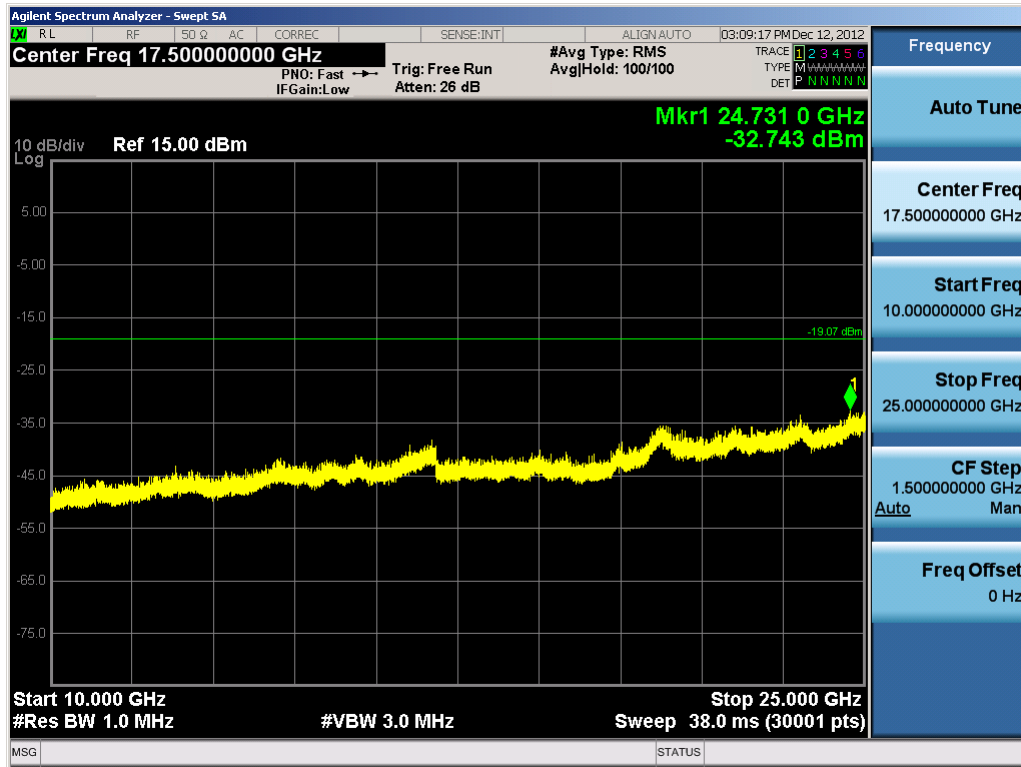
Plot 6-41. Conducted Spurious Plot (Bluetooth, 3Mbps – Ch. 78)
