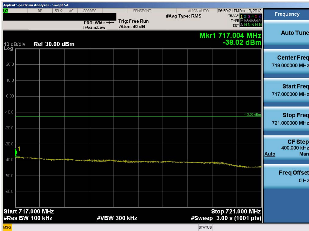
Plot 8-24. Upper Extended Band Edge Plot (10.0MHz QPSK – RB Size 50)
