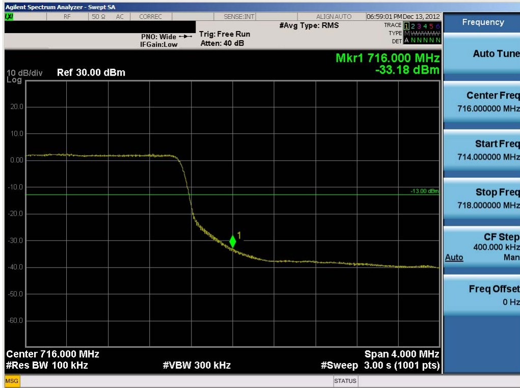
Plot 8-23. Upper Band Edge Plot (10.0MHz QPSK – RB Size 50)
